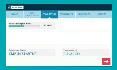
In order to ensure that the user can validate the committed performance and efficiency of these chillers, the new Blue Star brine chiller series is provided with advanced controllers that can display the capacity (TR) and chiller power consumption (kW) in real time. This unique feature not only enables users to validate the capacity and efficiency of each chiller but also helps optimise performance based on past data available in the controller.
