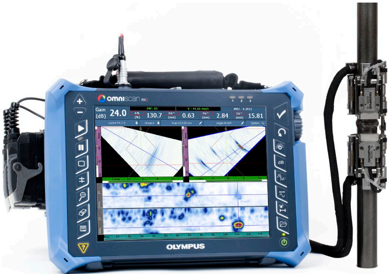
The COBRA scanner on a 0.84 in. OD pipe with two A15 PA probes with an OmniScan MX2 16:64 flaw detector displaying two PA groups with sectorial scans and C-scans.
