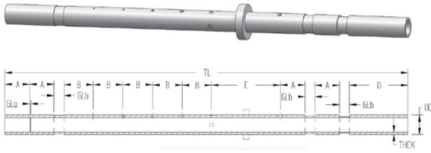
CT02 – ECT Extended ASME calibration tube.
