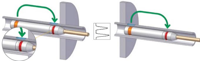
Large defect detected from the ABS channel on both sides of the support.
