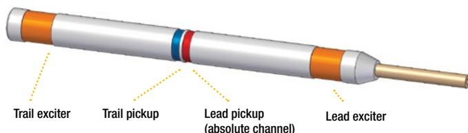
Dual-exciter probes can detect wear pits on both sides of the support plate, because there is always one exciter to supply energy to the pickup coils.
