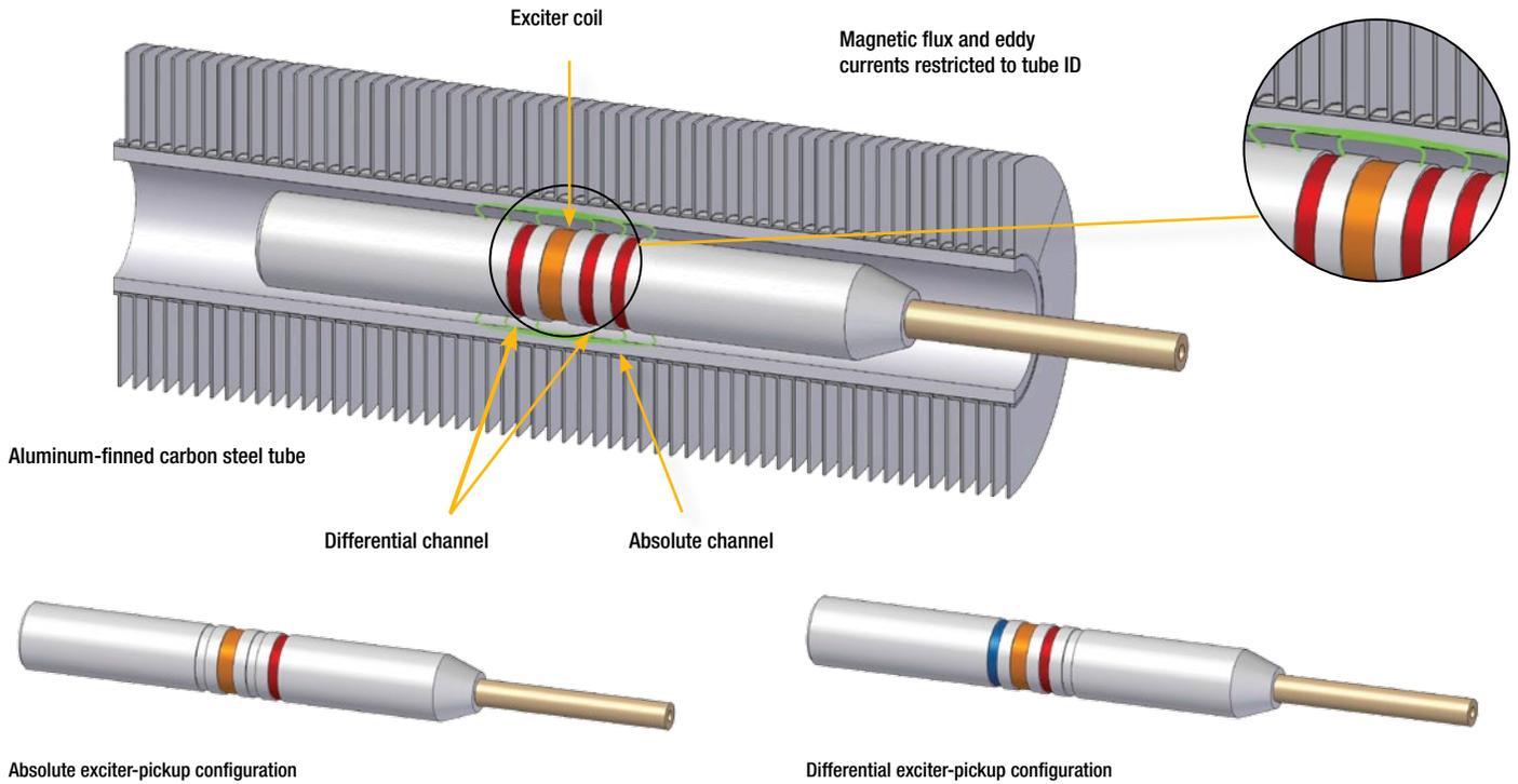
The Absolute channel easily detects internal volumetric defects, such as corrosion, erosion, and wall thinning. The damage severity can be evaluated by exclusively analyzing the signal amplitude.
