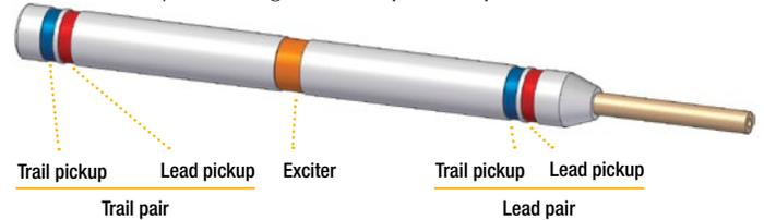
The dual pickup acts as two single-exciter probes in one probe casing, thus combining the excellent wall-loss response of the ABS channel with the dual-exciter model's capability to detect pits on each side of the support plate. This makes the dual-pickup model ideal for inspecting both tube sheets.
