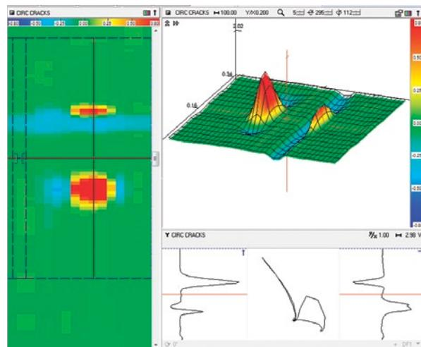
Circumferential cracks (75% and 50% at the support)
