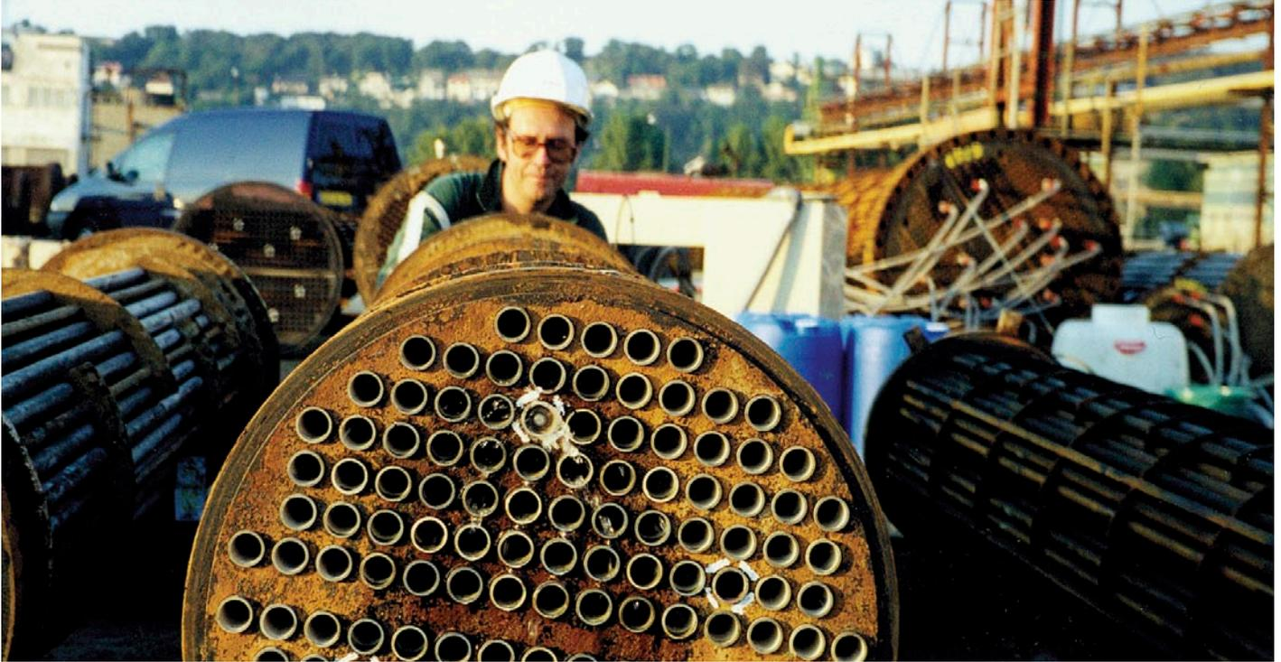
The internal rotary inspection system (IRIS) is an ultrasonic technique well suited to petrochemical and balance-of-plant (BOP) tube inspections. This technique uses an ultrasonic beam to scan the internal surface of the tube in helicoidal patterns, thus ensuring that the full length of the tube is tested. Olympus tube inspection systems monitor the front-wall and back-wall echoes to measure the tube wall thickness.
