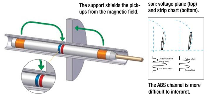
The short defect comparison: voltage plane (top) and strip chart (bottom).
