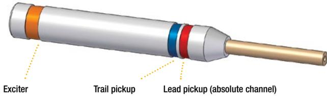
NOTE: The DIFF channel is made by subtracting the lead and trail pickups.
