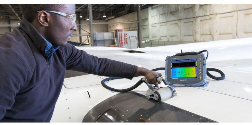
Olympus introduces the RollerFORM<sup>™</sup>, a new phased array wheel probe designed to address the inspection of composites and other smooth-surfaced materials. An affordable and easy-to-implement replacement for full 2-D encoding systems, the RollerFORM also offers a viable alternative to immersion techniques.
