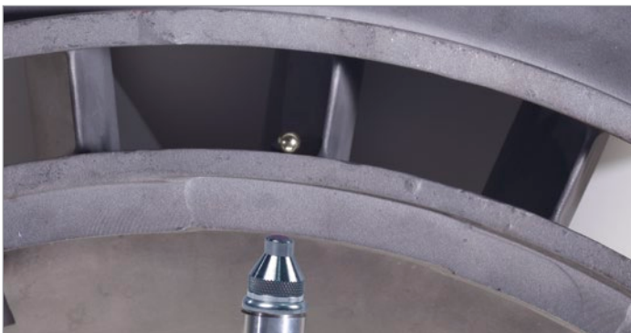
Measurement of a 24.1 mm (0.950 in.) aerospace casting
