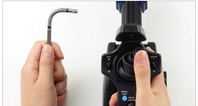
TrueFeel articulation providing a precise and controlled bend at the distal end
