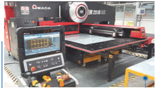
Fourth Turret Punching machine from Amada, Japan, installed at Blue Star's Wada Plant
