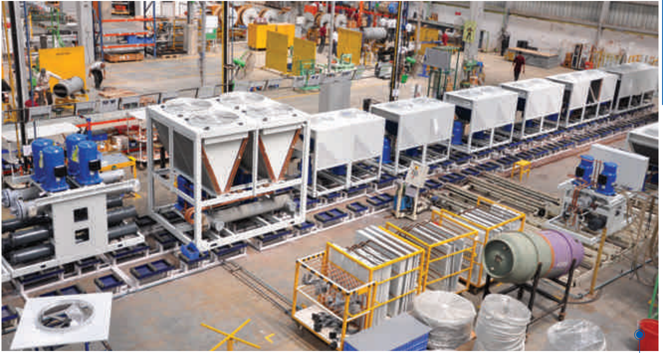
Scroll chiller assembly line at the Company's Wada manufacturing facility
