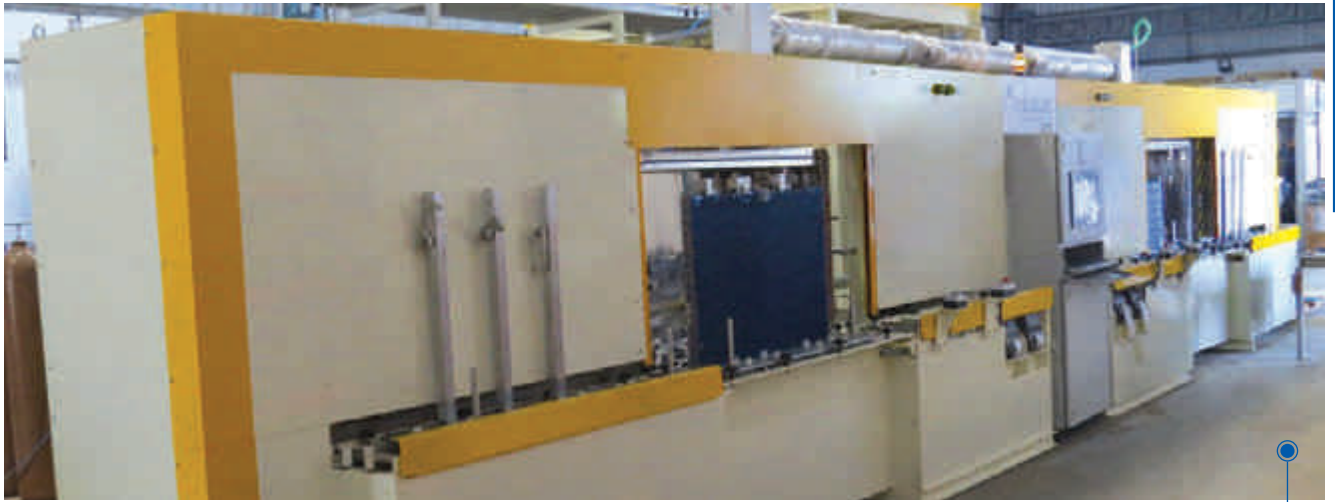
Helium leak detection machine installed at Blue Star's Himachal Pradesh Plant
