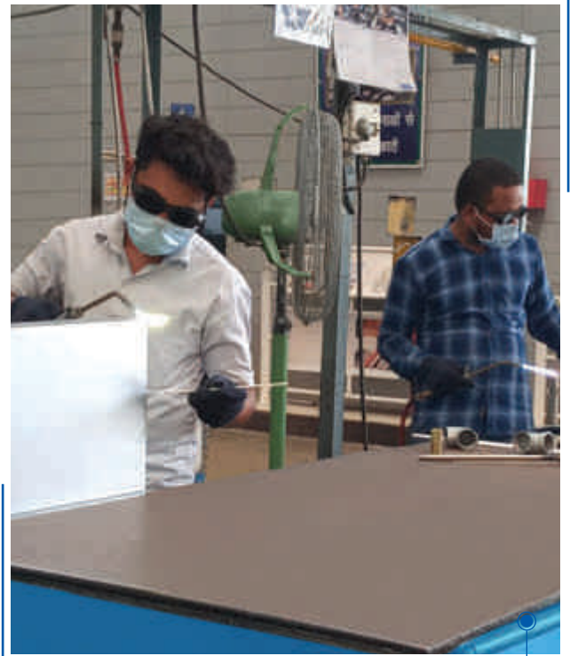
Deep tray welding work-in-progress at Blue Star's Dadra Plant
