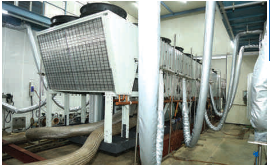
A glimpse of the AHRI certified air cooled chiller test lab
