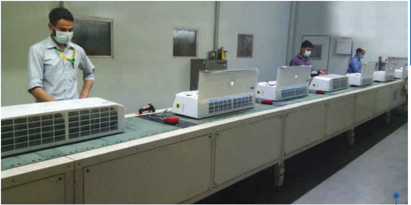
Inhouse indoor unit assembly line at Blue Star's Himachal Pradesh Plant
