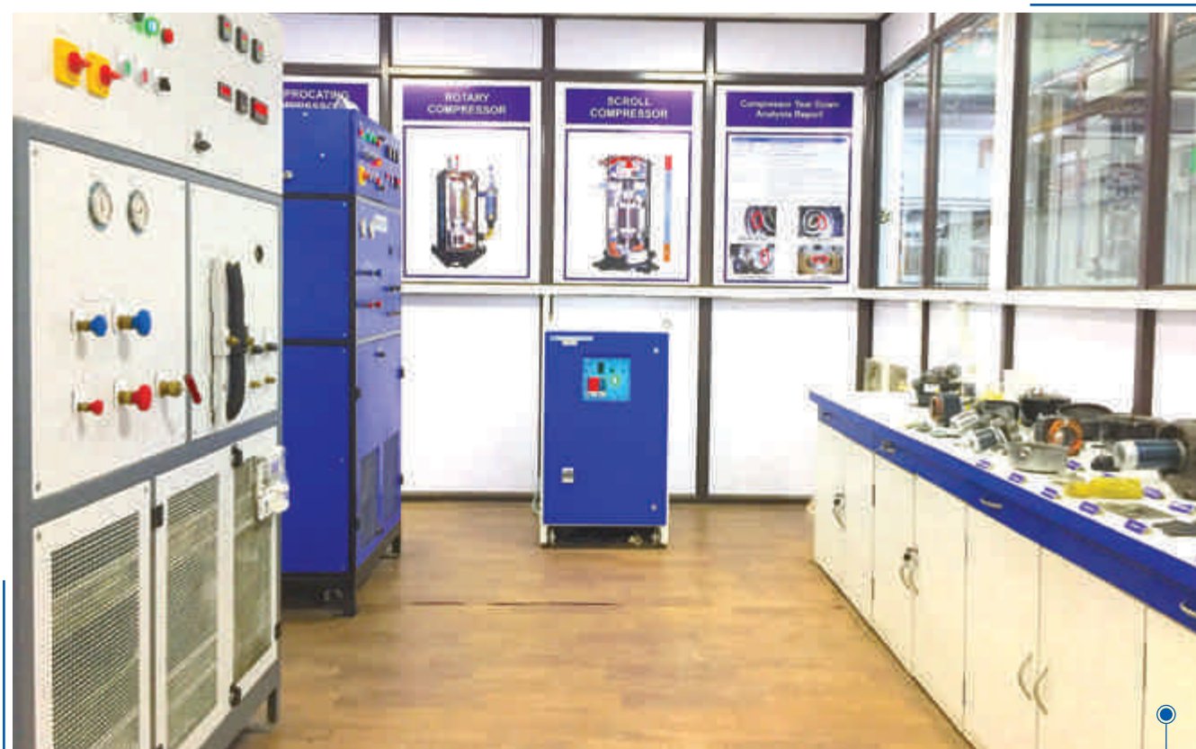
Compressor Lab comprising of two Compressor Test Rigs and Cut Sections of Tested Compressors at Blue Star's R&D facility in Thane
