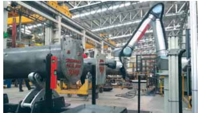
Collaborative Robot (COBOT) installed at Wada facility
