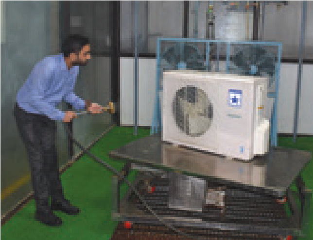
A water Ingress Protection (IP) test being conducted at Blue Star's R&D facility
