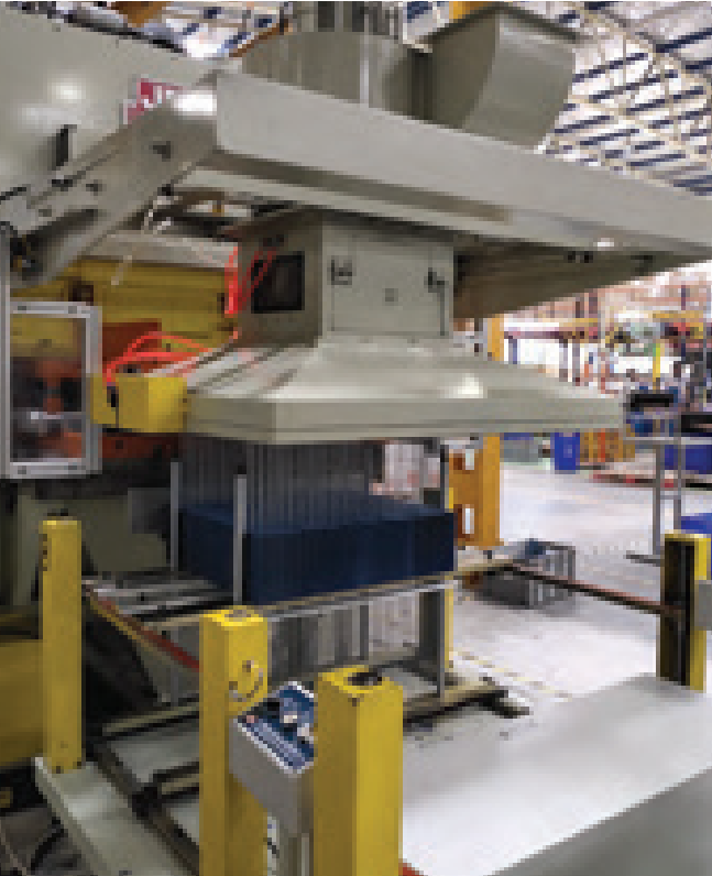
The 5 mm Fin Press and Vertical expander machines were installed at the Himachal Pradesh Plant to produce the recommended 5 mm coils, which are used in some models instead of the older 7 mm coils
